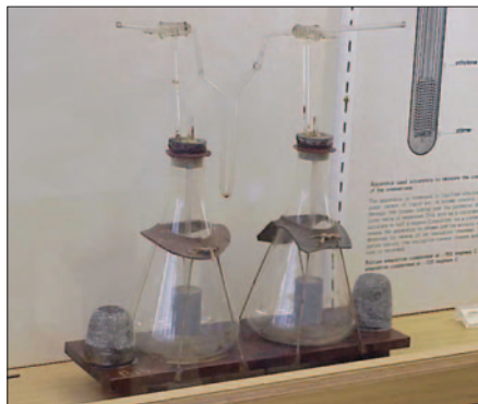
Figure 8. In one of his pioneering researches, Rutherford first demonstrated the prodigious amount of heat generated by radioactivity. Using this differential air calorimeter (where two flasks were connected by a manometer), a known mass of radium is inserted in the right flask and a resistance wire in the left flask. The heat was adjusted in the resistance wire on the left so that xylene in the manometer (indicating relative pressure in the two flasks) is balanced by equally heated air in both flasks. The amount of heat generated by the radium (1 gram) was calculated to be 110 gram-calories/hour, enormously greater than that generated in chemical reactions. Rutherford expanded this experiment to separate out the contributions of gamma radiation (using lead shielding) and emanation (by purging of the flasks).
